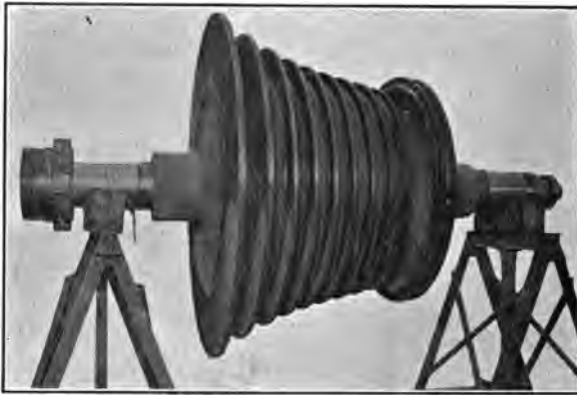
FIG. 80.—U. S. S. California : View of Assembled Turbine Rotor for Propulsion Unit No. 1
